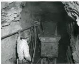
Loading car in uranium mine. Scoop dumping ore into car in part of a mechanical loader operated on compressed air brought into the mine by the pipe at left. (1983.63.178)
