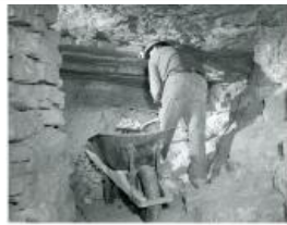
Hand loading ore into a wheelbarrow (1983.63.73)
