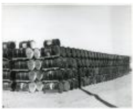
Vanadium storage looking Northwest - 55 drums comparatively new (note rust on bottom and stacking arrangement (18 Feb 1958) (1983.63.160)
