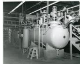
Alkaline Leach Autoclave - Pilot Plant, Grand Junction (1983.63.136)
