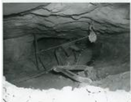
Drilling blast holes in thin-bedded uranium ore, with scraper in foreground (1983.63.177)
