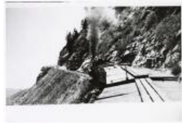
Uintah locomotive climbing 7.5% grade on Baxter Pass. (1987.39.5)
