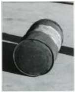
A typical old drum found to be corroded to the point it was leaking (18 Feb 1958) (1983.63.162)
