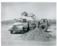
Loading uranium ore into truck at government ore-buying station and sampling plant (1983.63.190)
