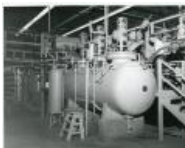
Alkaline Leach Autoclave - Pilot Plant, Grand Junction (1983.63.136)
